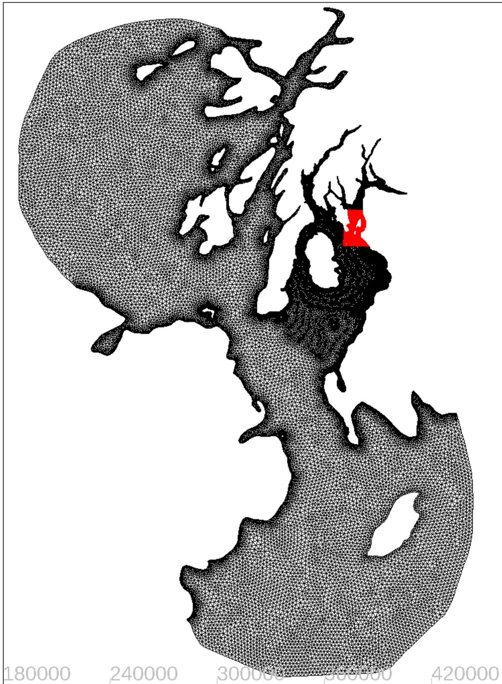
**Figure 2** *Computational mesh – red zone represents the area of focus around Little Cumbrae (see Section 2.3).*
