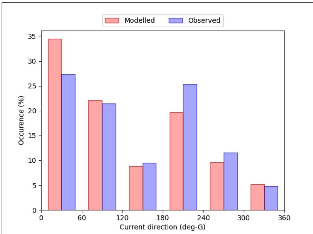
**Figure 12** Histogram of observed and modelled current direction from 4<sup>th</sup>-26<sup>th</sup> October 2017 (near-surface measurement point – see Figure 1). Model skill  $d2 = 0.96$ .
