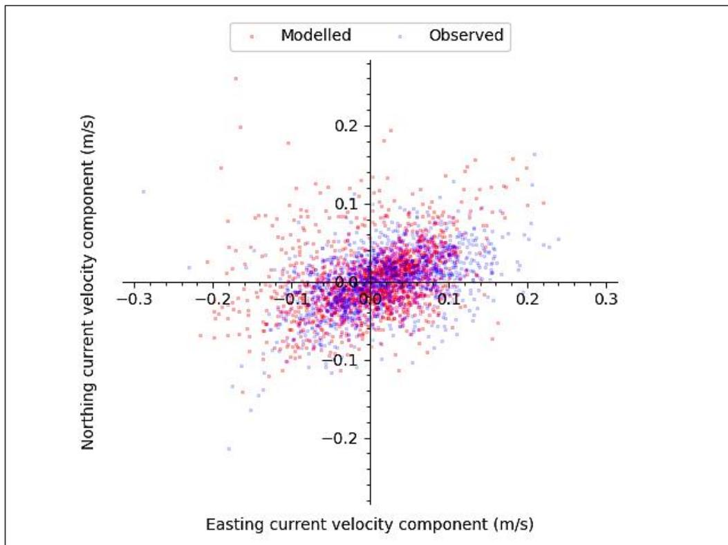
**Figure 20** Scatter plot of observed and modelled velocity from 4<sup>th</sup>-26<sup>th</sup> October 2017 (near-bottom measurement point – see Figure 1).
