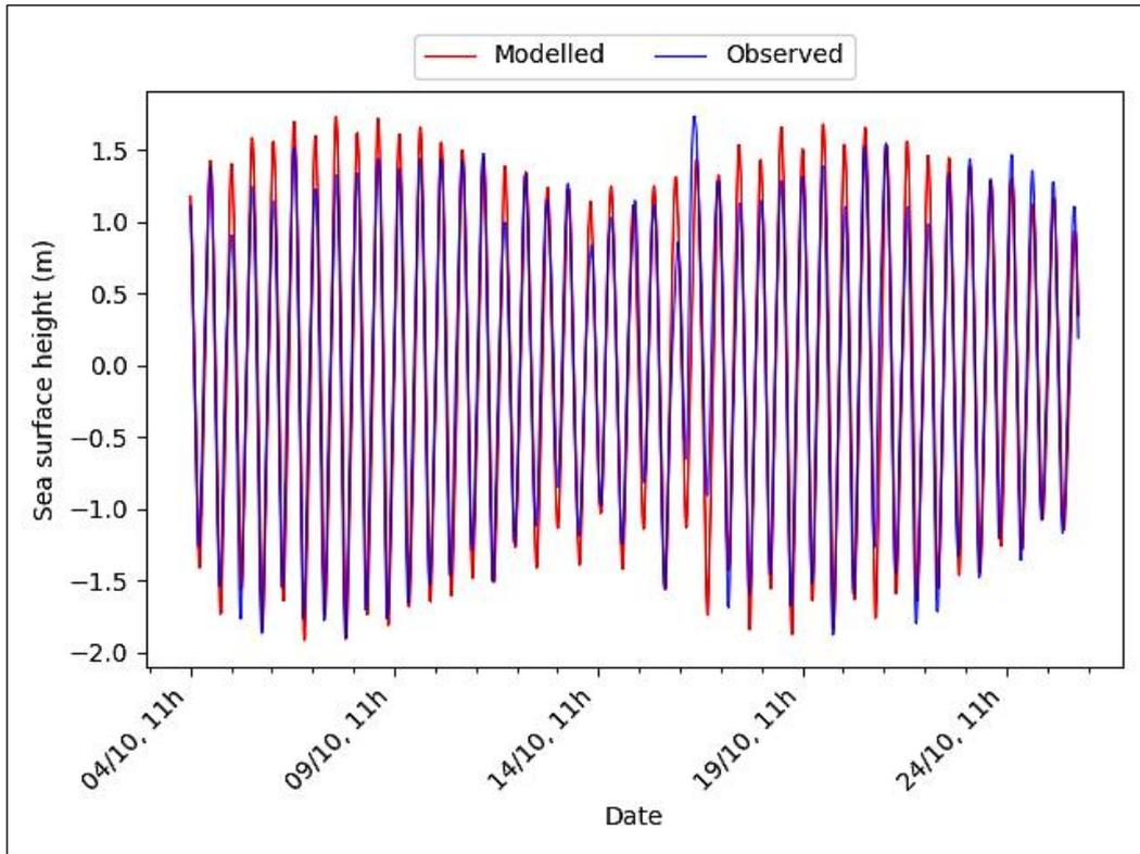
**Figure 19** Comparison between observed and modelled sea surface height from 4<sup>th</sup>-26<sup>th</sup> October 2017 (near-bottom measurement point – see Figure 1).
