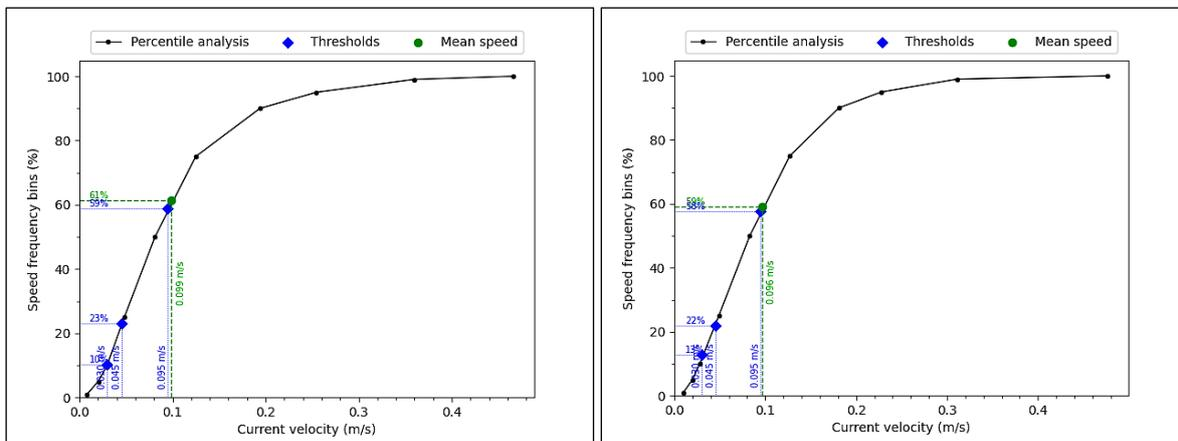
**Figure A.4** Current speed (m/s) percentile analysis for the near-surface measurement point. Telemac model (left) and observation (right).
