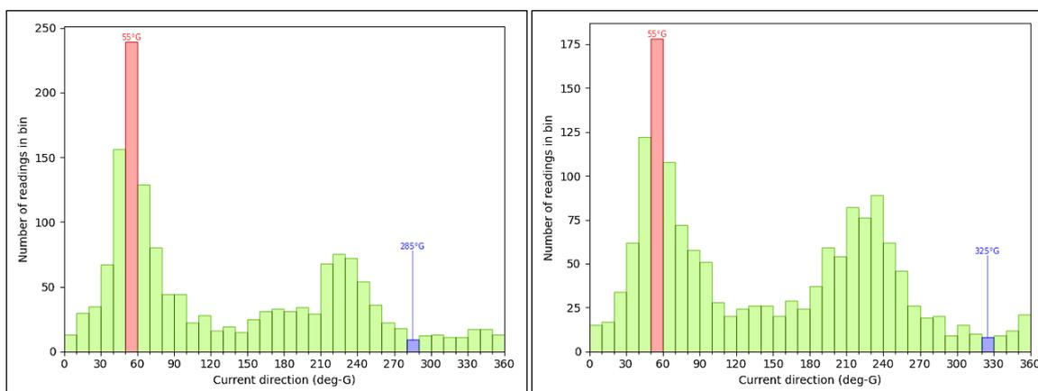
**Figure A.2** Current direction bar graph (deg) for the near-surface measurement point. Telemac model (left) and observation (right).
