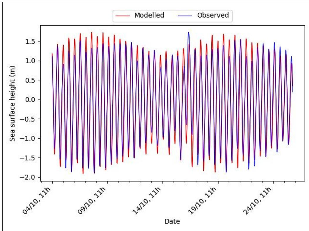
**Figure 13** Comparison between observed and modelled sea surface height from 4<sup>th</sup>-26<sup>th</sup> October 2017 (mid-height measurement point – see Figure 1).
