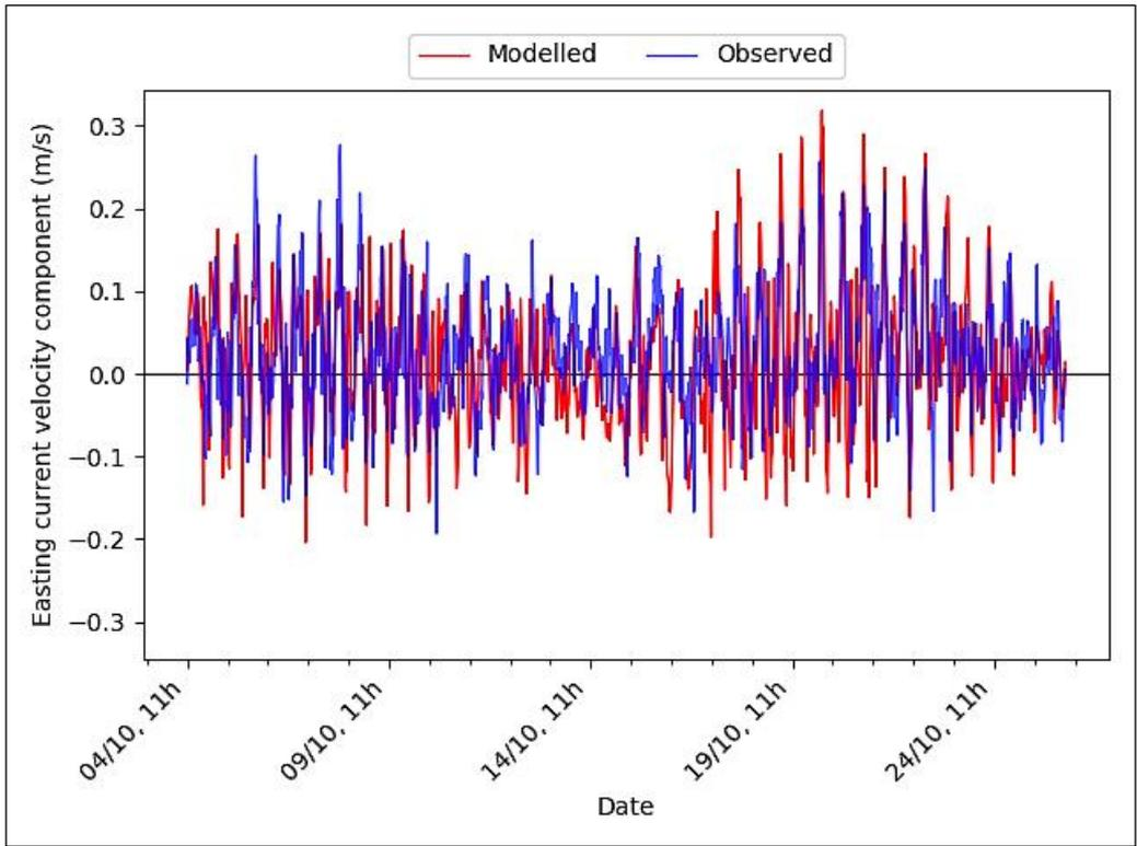
**Figure 15** Comparison between observed and modelled East velocity component from 4<sup>th</sup>-26<sup>th</sup> October 2017 (mid-height measurement point – see Figure 1).
