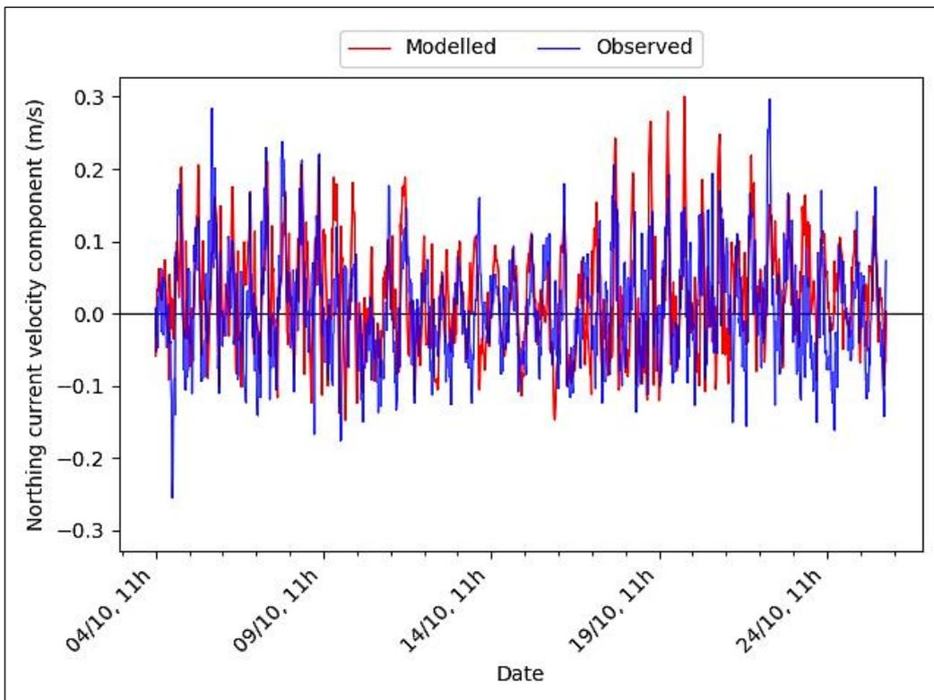
**Figure 10** Comparison between observed and modelled North velocity component from 4<sup>th</sup>-26<sup>th</sup> October 2017 (near-surface measurement point – see Figure 1).
