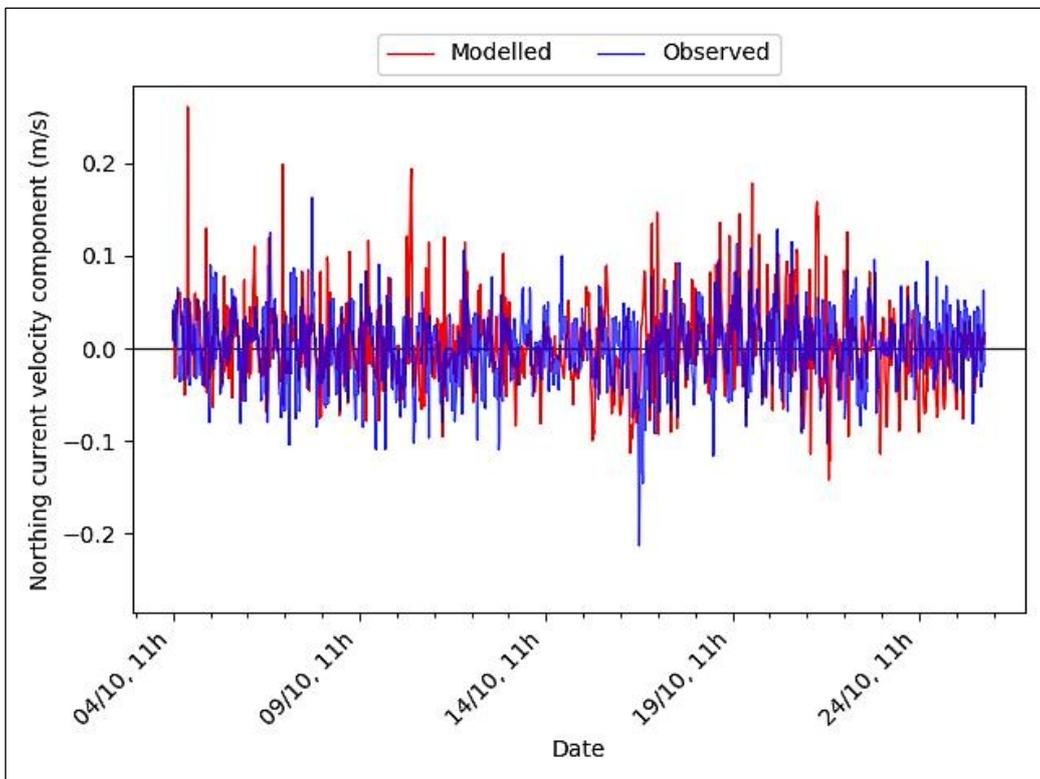
**Figure 22** Comparison between observed and modelled North velocity component from 4<sup>th</sup>-26<sup>th</sup> October 2017 (near-bottom measurement point – see Figure 1).
