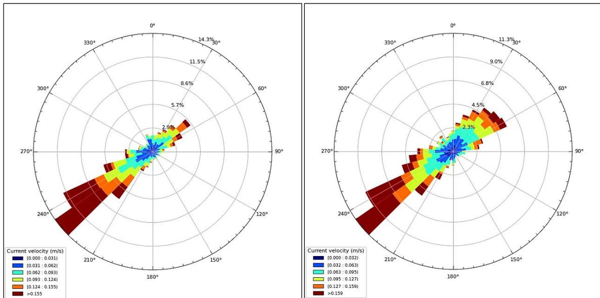
**Figure A.5** Filled wind rose of current velocity (m/s) for the near-surface measurement point. Telemac model (left) and observation (right).
