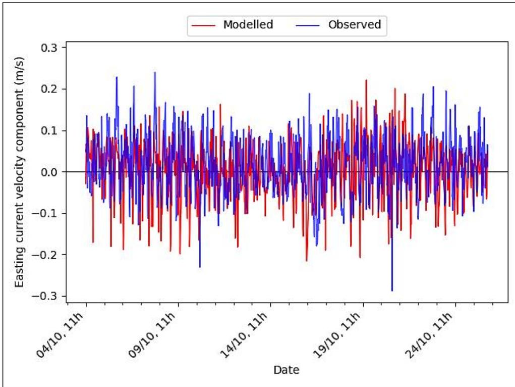
**Figure 21** Comparison between observed and modelled East velocity component from 4<sup>th</sup>-26<sup>th</sup> October 2017 (near-bottom measurement point – see Figure 1).
