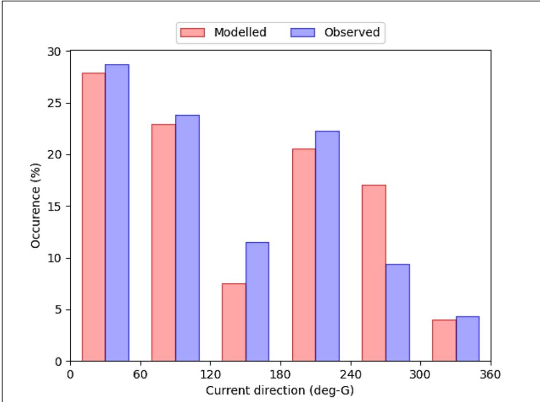
**Figure 18** Histogram of observed and modelled current direction from 4<sup>th</sup>-26<sup>th</sup> October 2017 (mid-height measurement point – see Figure 1). Model skill  $d_2 = 0.95$ .
