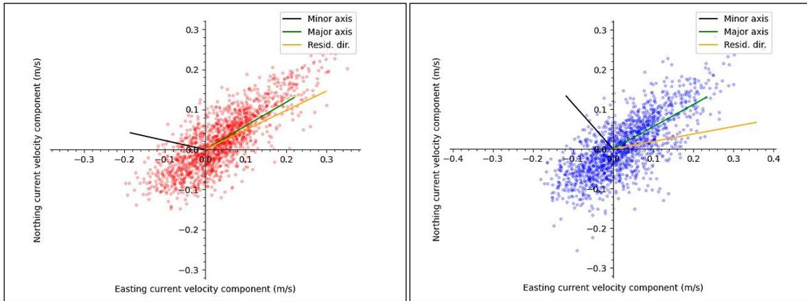
**Figure A.3** Easting versus northing velocity component (m/s) for the near-surface measurement point. Telemac model (left) and observation (right).
