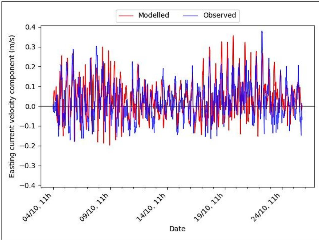
**Figure 9** Comparison between observed and modelled East velocity component from 4<sup>th</sup>-26<sup>th</sup> October 2017 (near-surface measurement point – see Figure 1).
