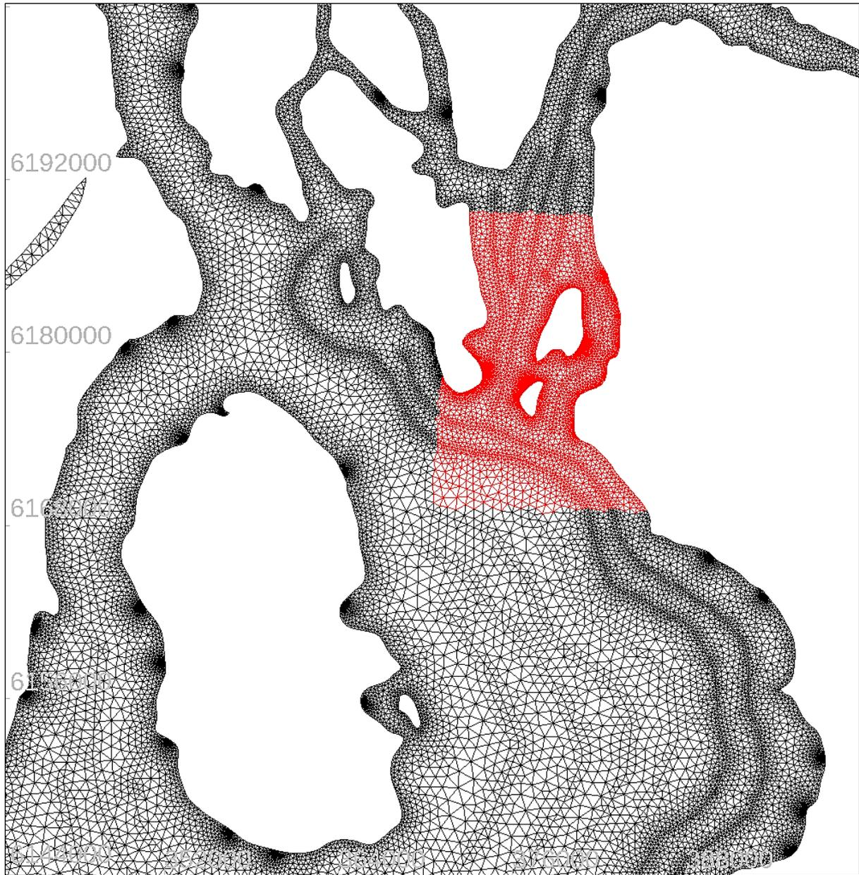
**Figure 5** *Zoomed view of the original Telemac 3D hydrodynamics mesh (38.2 Gb, black) and the reduced size model (3.1 Gb, red). Denser mesh areas on the coastline show approximate river inlet locations.*
