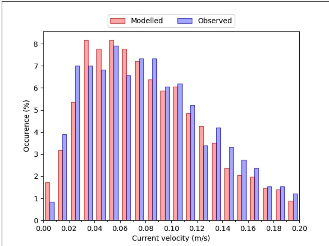
**Figure 11** Histogram of observed and modelled current speed component from 4<sup>th</sup>-26<sup>th</sup> October 2017 (near-surface measurement point – see Figure 1). Model skill  $d2 = 0.97$ .
