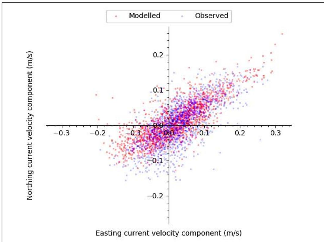
**Figure 14** Scatter plot of observed and modelled velocity from 4<sup>th</sup>-26<sup>th</sup> October 2017 (mid-height measurement point – see Figure 1).
