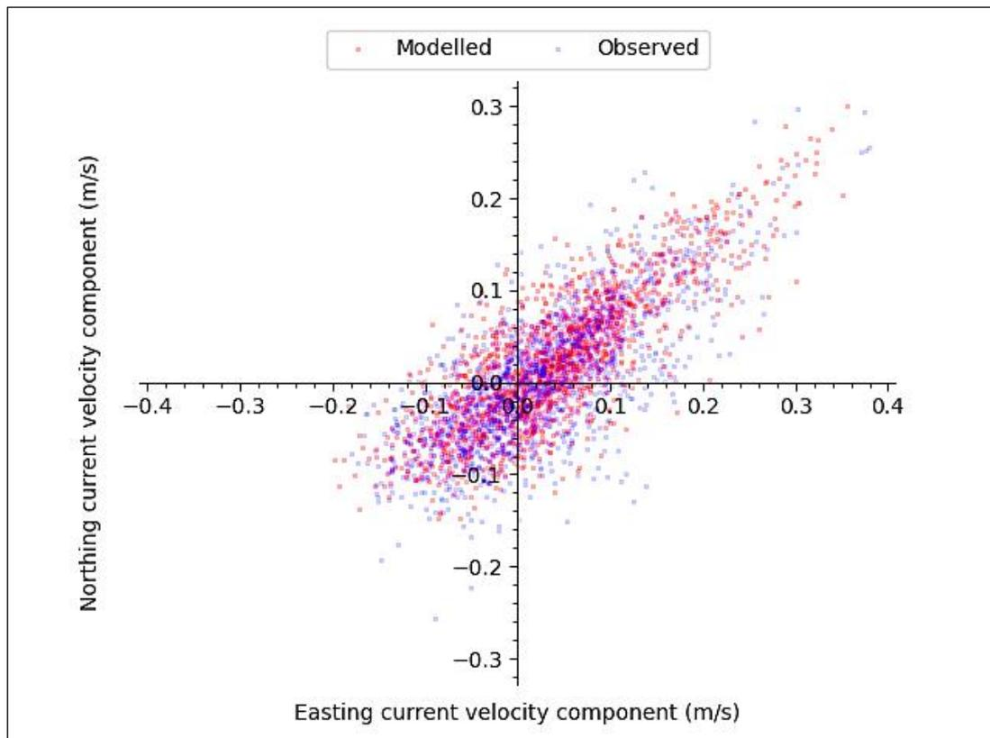
**Figure 8** Scatter plot of observed and modelled velocity from 4<sup>th</sup>-26<sup>th</sup> October 2017 (near-surface measurement point – see Figure 1).
