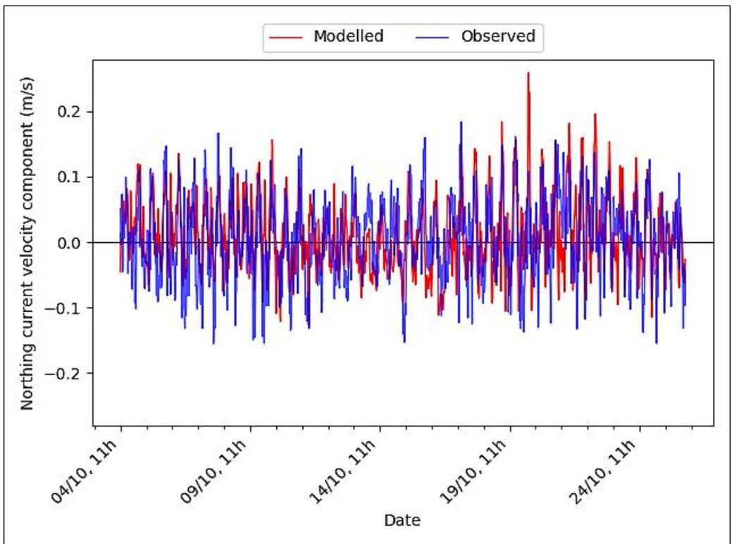
**Figure 16** Comparison between observed and modelled North velocity component from 4<sup>th</sup>-26<sup>th</sup> October 2017 (mid-height measurement point – see Figure 1).
