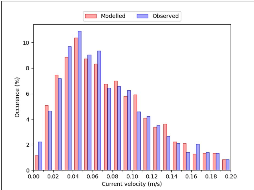
**Figure 17** Histogram of observed and modelled current speed component from 4<sup>th</sup>-26<sup>th</sup> October 2017 (mid-height measurement point – see Figure 1). Model skill  $d_2 = 0.99$ .
