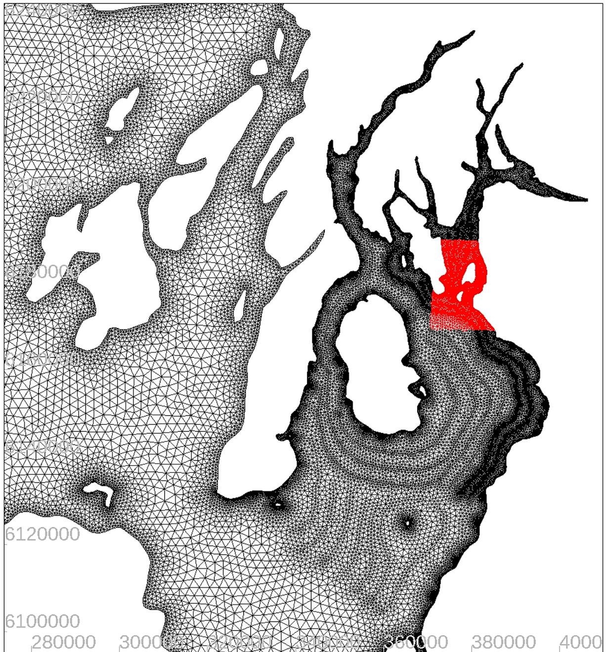
**Figure 4** Zoomed view of the original Telemac 3D hydrodynamics mesh (38.2 Gb, black) and the reduced size model (3.1 Gb, red).
