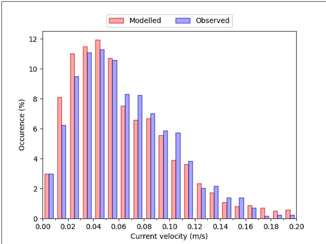
**Figure 23** Histogram of observed and modelled current speed component from 4<sup>th</sup>-26<sup>th</sup> October 2017 (near-bottom measurement point – see Figure 1). Model skill  $d_2 = 0.99$ .
