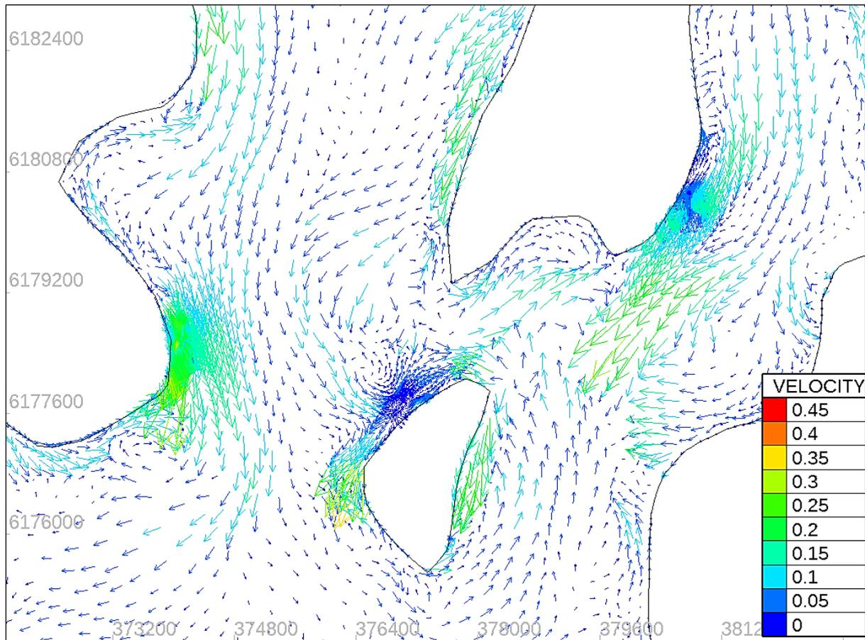
**Figure 26** Velocity vectors (m/s) in the near-sea bed layer around Little Cumbrae on the 25<sup>th</sup> October 2017 at 08h40.
