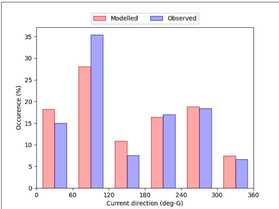
**Figure 24** Histogram of observed and modelled current direction from 4<sup>th</sup>-26<sup>th</sup> October 2017 (near-bottom measurement point – see Figure 1). Model skill  $d_2 = 0.95$ .
