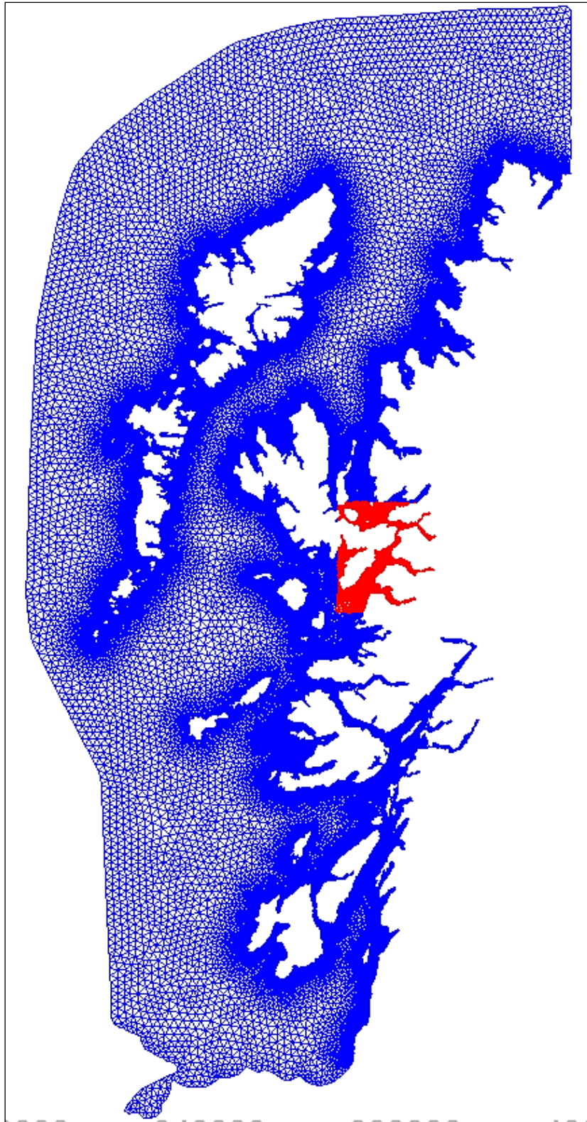
Figure 23 Original Telemac 3D hydrodynamics mesh (36 Gb, blue) and reduced size model (2.6 Gb, red).
